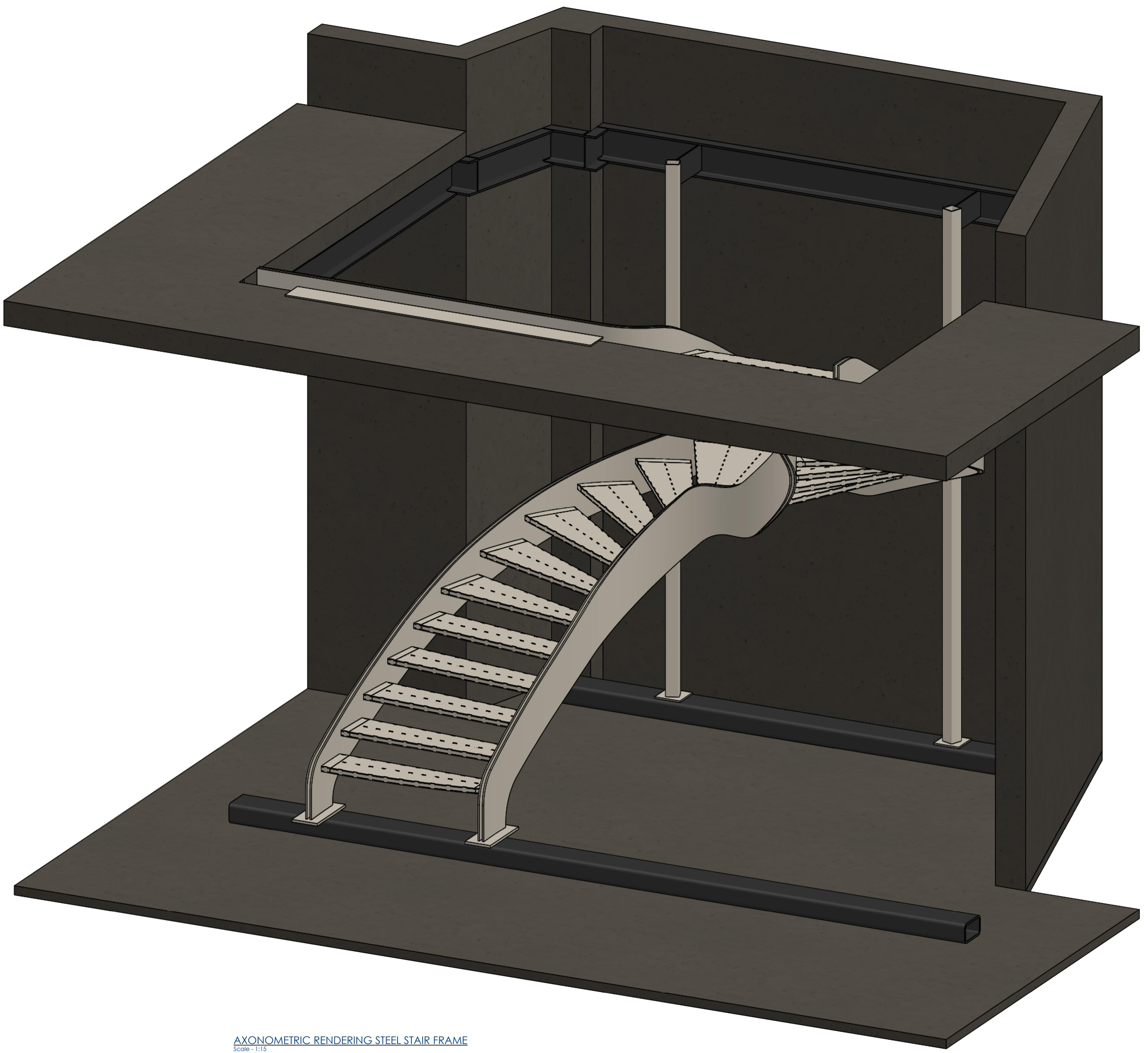
AXONOMETRIC RENDERING STEEL STAIR FRAME
