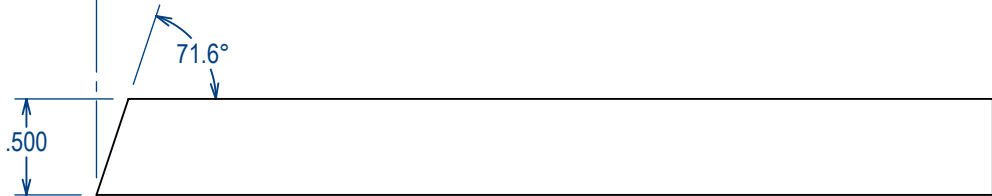
Side Face - Part #WH9 Scale - 1:1 Material: Stainless Steel 304 Body Section: 0.5x2 Finish: Blackened per Approved Sample Quantity: 2
